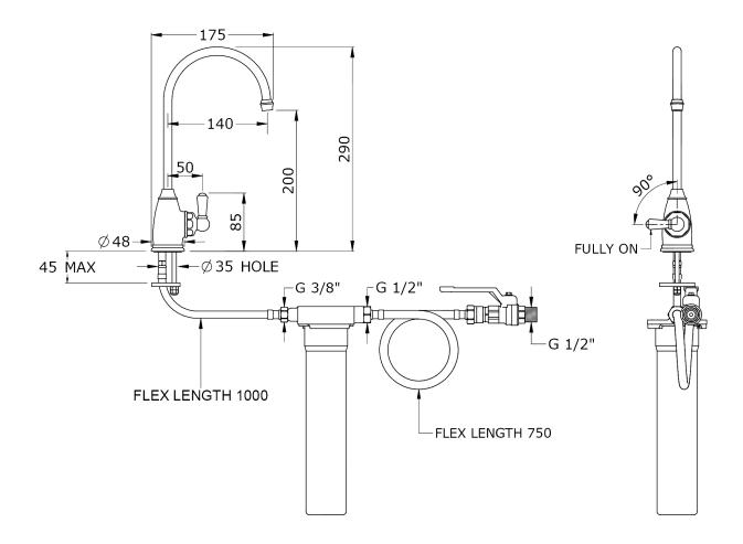
Temp Range Min 1°C / 34°F Recommended Min 1 bar / 15 psi Max 70°C / 158°F Working Pressure Max 5 bar / 75 psi
